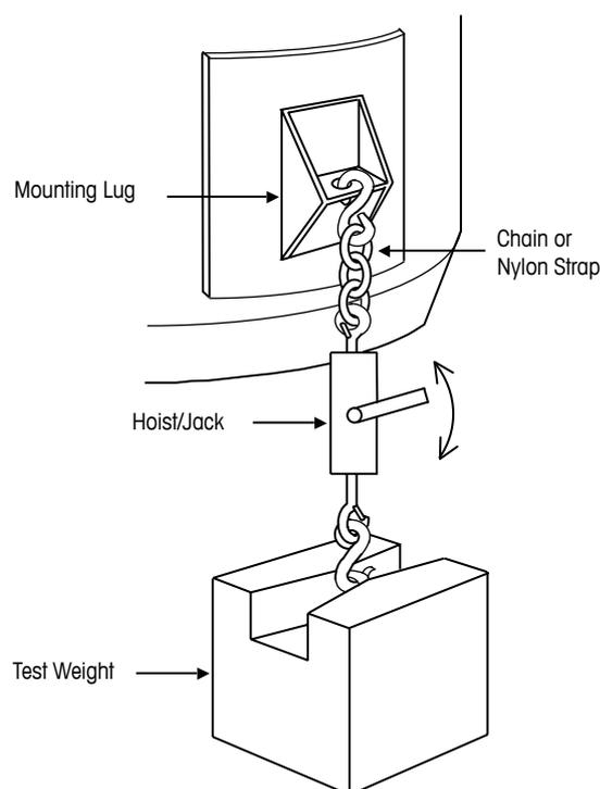
Calibrating a tank with mass traceable to a standard.
