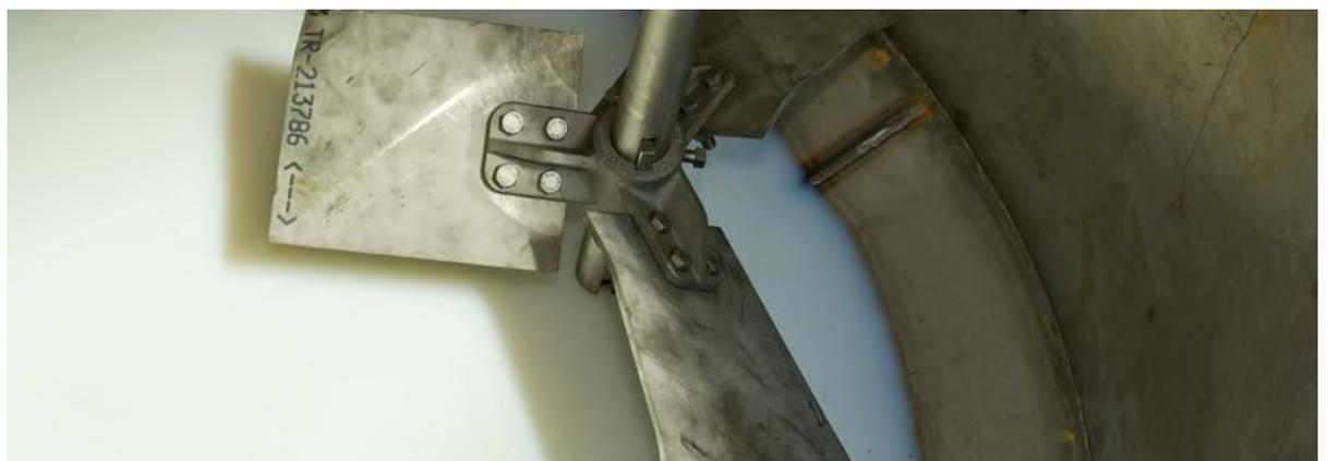
Above is a look into a tank with a mixer for paint manufacturing. Installations, such as mixers, wave breakers or heaters might complicate accurate measuring with level sensors.
