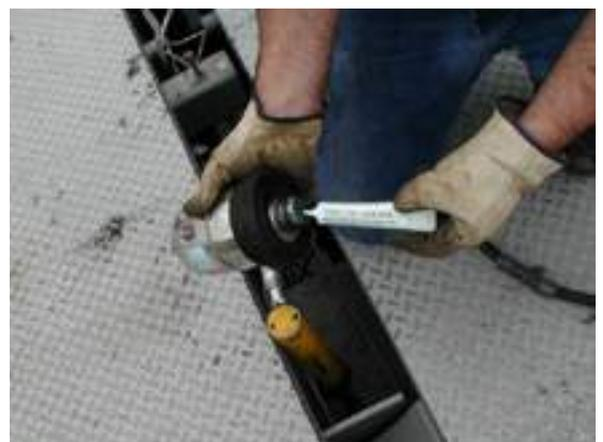
Some areas, such as load cell mating surfaces, require periodic lubrication
