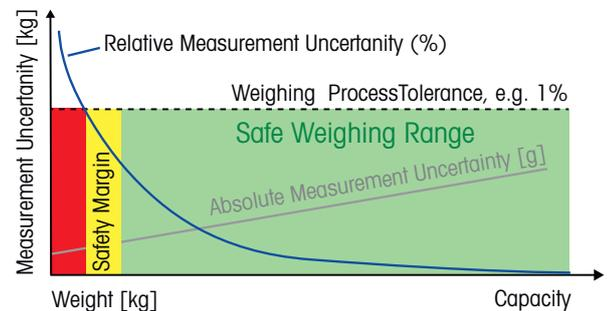
Figure 2: Measurement Uncertainty and Safe Weighing Range
